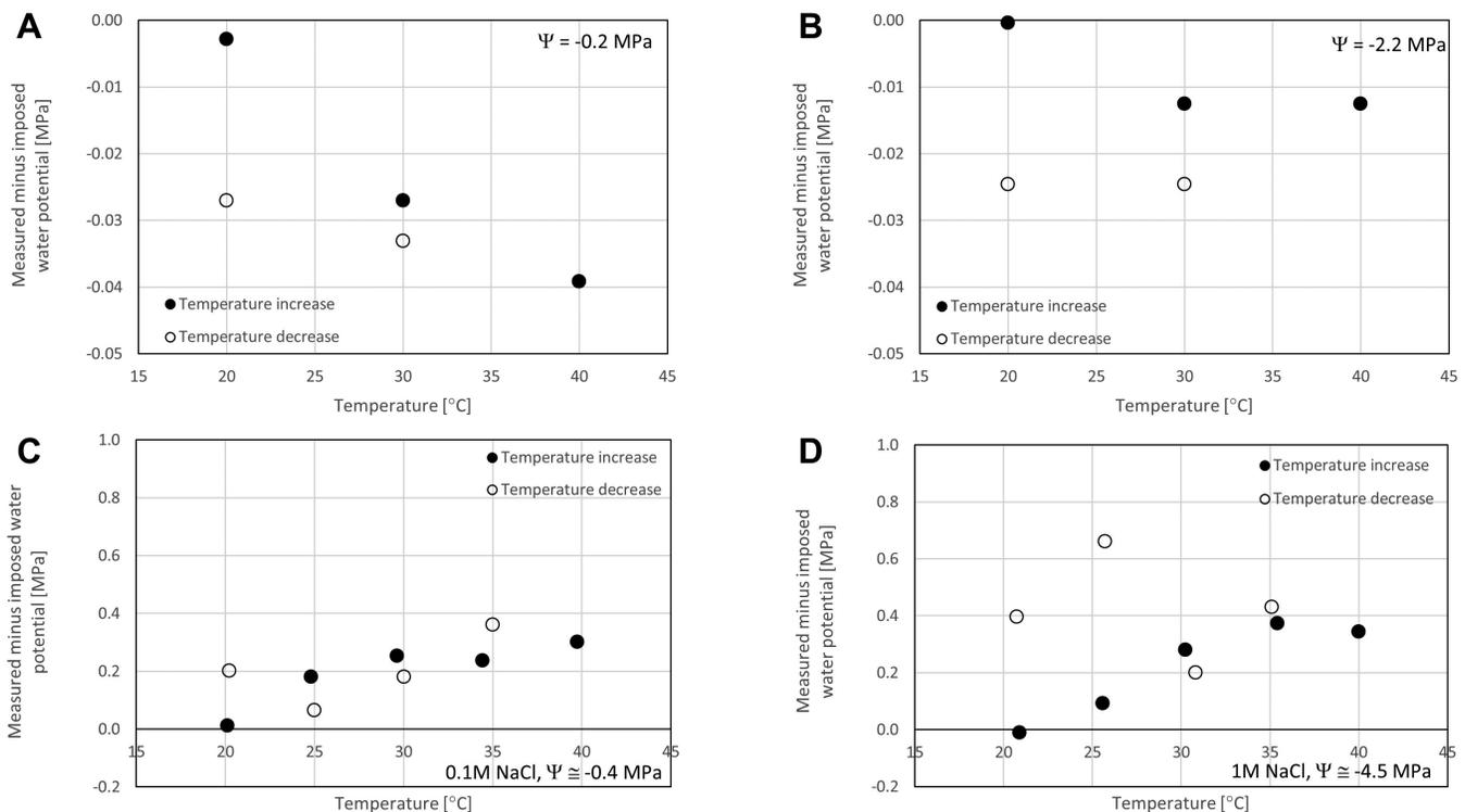
**Fig. 3.** (A, B) Effect of temperature on HCT measurement: (A) imposed water potential  $\Psi=0.2$  MPa; (B) imposed water potential  $\Psi=2.2$  MPa. (C, D) Effect of temperature on TP measurement: (C) imposed water potential  $\Psi \approx -0.4$  MPa (0.1 M NaCl solution); (D) imposed water potential  $\Psi \approx -4.5$  MPa (1 M NaCl solution).
