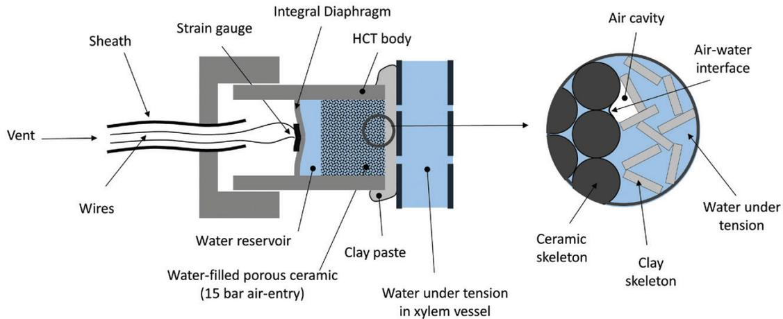
Fig. 2. High-capacity tensiometer (after Tarantino and Mongioli, 2002).
