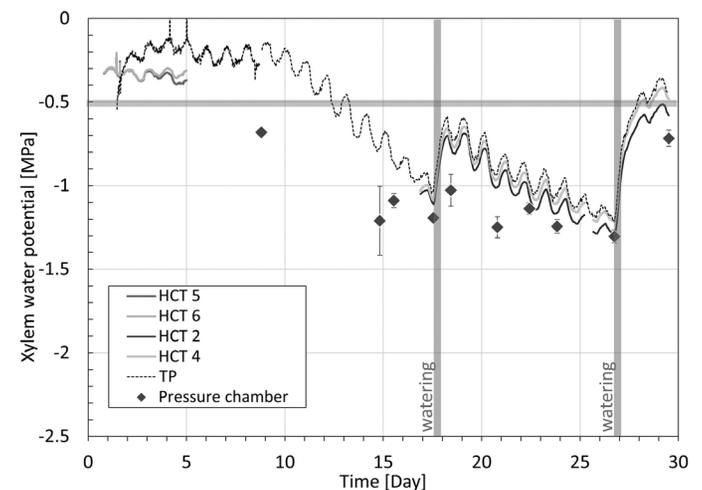
**Fig. 5.** Measurement of xylem water pressure by the HCT and TP, and by the pressure chamber on non-transpiring leaves, on the cherry sapling. The measurements made with the different HCTs and the TP are indicated by the different curves. For the pressure chamber measurements, grey diamonds represent the average values and the error bars represent the SD. The vertical grey bands indicate watering times. The horizontal grey line marks the value of  $-0.5$  MPa xylem water potential.
