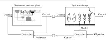
Fig. 1. Control hierarchy of the crop-treatment system.
