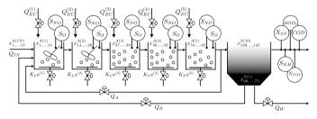
Fig. 3. The activated sludge plant: Process layout.
