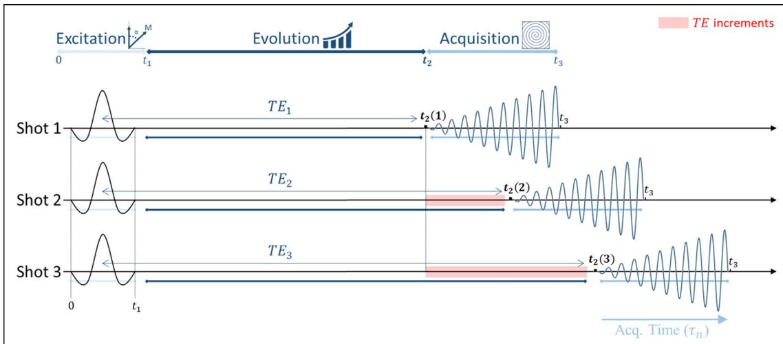
**Fig. 1.** Illustration of the IDEAL spiral spectral encoding scheme. It consists of radiofrequency (RF) pulses applied during an excitation time ( $t_1$ ), and an acquisition with spiral spatial encoding ( $t_3 - t_2$ ) applied after an evolution time ( $t_2(m) - t_1$ ). Several shots with different evolution times are used to encode the spectral information.
