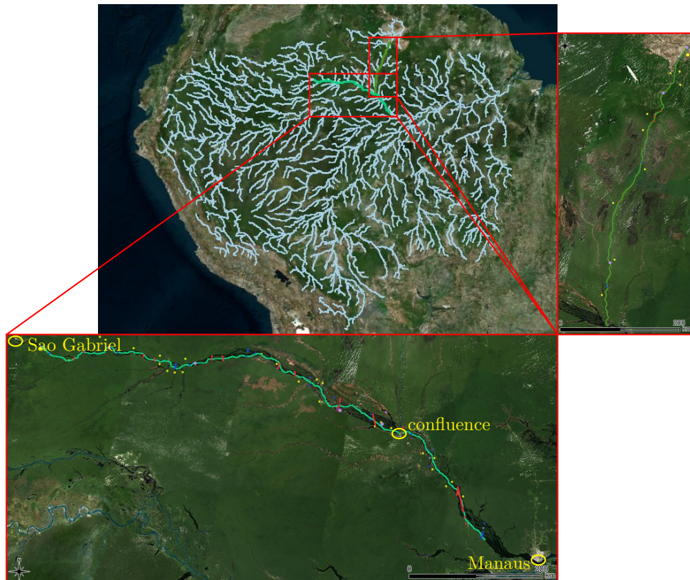
Figure 1 – Study zone and observability: the Negro-Branco River network in the Amazon basin with hydrological inflow points in yellow, and multi-mission virtual stations locations - S3A stations in blue, S3B stations in red and J3 stations in purple.
