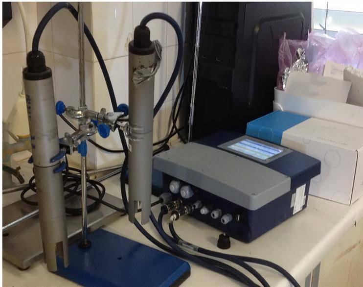
**Figure 5.8** Dissolved N<sub>2</sub>O probes with protective cover (left), and measurement controller (right). Photo courtesy of Dr. Adrian Oehmen (The University of Queensland).
