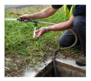
**Figure 5.2** Collection of dissolved  $CH_4$  sample directly from the rising main into an airtight syringe, adapted from Foley *et al.* (2009). Reprinted from Water Science & Technology, volume 60, issue number 11, pages 2963–2971, with permission from the copyright holders, IWA Publishing.
