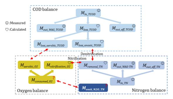
**Figure 5.9** Simplified illustration of the methodology to determine the N<sub>2</sub>O volumetric transfer coefficient via oxygen mass balance analysis.
