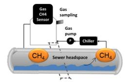
**Figure 5.4** A purpose-built device for gas sampling or infrared (IR) gas sensor application in sewer headspace: a gas pump continuously recycles the gas from the sewer headspace to the chamber and then back to the sewer. A chiller is used in the gas line feeding the chamber to maintain the desired level of 50–70% relative humidity (RH) for the IR sensor (adapted from Liu *et al.*, 2015a).
