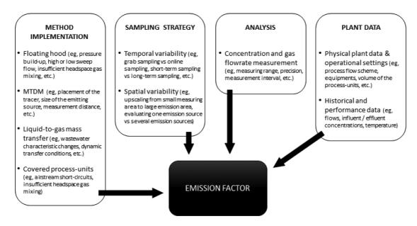
Figure 5.10 Potential sources of errors impacting the estimation of GHG emission factors at WWTPs.
