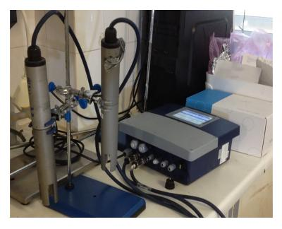
**Figure 5.8** Dissolved  $N_2O$  probes with protective cover (left), and measurement controller (right). Photo courtesy of Dr. Adrian Oehmen (The University of Queensland).
