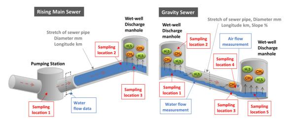
**Figure 5.1** Sampling points and data required to quantify  $CH_4$  emissions depending on the typology of sewer (adapted from Liu *et al.*, 2015a).
