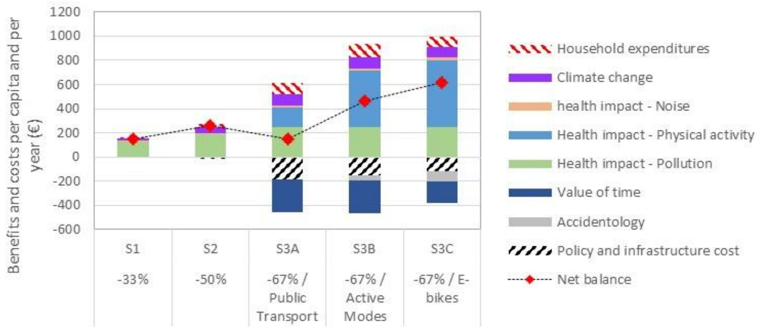
Figure 7. Result of the cost-benefit analysis per year and per capita for each scenario. The overall gain is shown by the red diamond shape while surfaces indicate the structure of costs and benefits.
