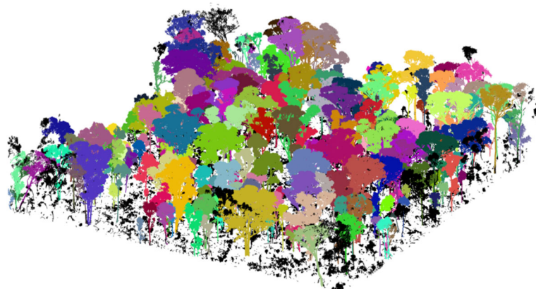
Fig. 6 Extracted individual trees. Each tree is colored randomly, and black color indicates non-tree objects
