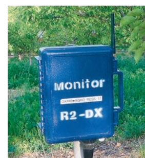
2 Tensiometers and monitor used for monitoring the availability of water in the soil.
