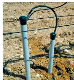
2 Tensiometers and monitor used for monitoring the availability of water in the soil.
