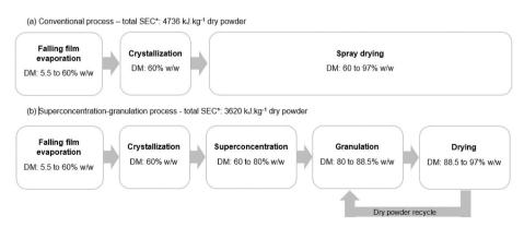
**Fig. 1.** Schematic representation for the manufacture of whey permeate powder (a) conventional spray drying and (b) novel superconcentration-granulation process for manufacture of whey permeate powder (WPP). DM, Dry matter; SEC, Specific energy consumption for dehydration (kJ.kg<sup>-1</sup> dry powder); \*Energy estimates from the study of Tanguy et al. (2017).
