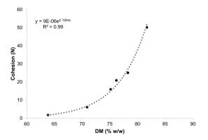
Fig. 7. Cohesion (in N) as a function of DM of superconcentrates (% w/w). Measurements at 25  $^{\circ}$ C. Standard deviation less than 3% (n = 2), error bars are within the symbols.
