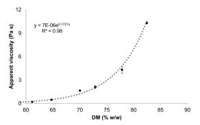
**Fig. 4.** Apparent viscosity of superconcentrates as a function of dry matter (DM). Measurement at 25  $^{\circ}\text{C}$  and 100 s $^{-1}$ . Error bars represent standard deviation of measurements performed in duplicates.
