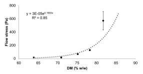
**Fig. 6.** Flow stress (Pa) using oscillation amplitude sweep as a function of dry matter of superconcentrates (% w/w). Measurement made at 60 °C and constant frequency of 1 Hz. Error bars represent standard deviation (n = 2).
