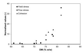
**Fig. 8.** Comparison of the three rheological techniques based on normalized results of yield stress (Herschell-Bulkley model), flow stress (oscillation amplitude sweep) and cohesion (probe track test) as a function of DM content of superconcentrates (% w/w). Values were normalized on Y-axis with respect to the value corresponding to DM on x-axis.
