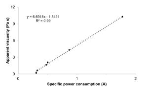
**Fig. 5.** Correlation of apparent viscosity of superconcentrates (Pa s) and specific power consumption of mixer expressed as current (A). Viscosity measurement made at  $25\,^{\circ}$ C and  $100\,\text{s}^{-1}$ . Agitation speed of 500 rpm. Correlation is based on average values of apparent viscosity (n = 2).
