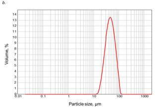
Fig. 3. a. Desupersaturation curve of MFP during crystallization at 60% w/w 30 °C. (Lactose g.g $^{-1}$  water – open circles; Extent of crystallization – dark circles); b. Particle size of the lactose crystals measured using laser light diffraction.
