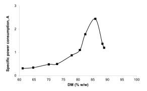
Fig. 10. Specific power consumption of mixer expressed in ampere (A) as a function of dry matter (DM) of superconcentrates. Experiments carried out at 500 rpm and 60  $^{\circ}$ C.
