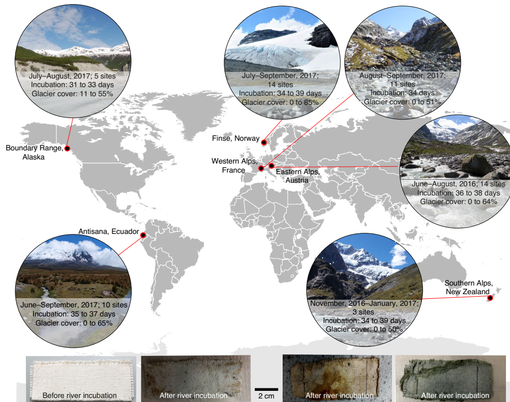
Fig. 1 | Global distribution and experimental details of glacierized mountain river sampling sites. For each sampling region, the date and duration of cotton-strip incubation are displayed alongside the number of river sites sampled and the range of percentage catchment glacier cover that they represent. The cotton-strip images display examples of before versus after incubation. Further site information is provided in Supplementary Table 1. Photograph of Antisana, Ecuador, is adapted with permission from ref. 45 , Springer Nature Limited.
