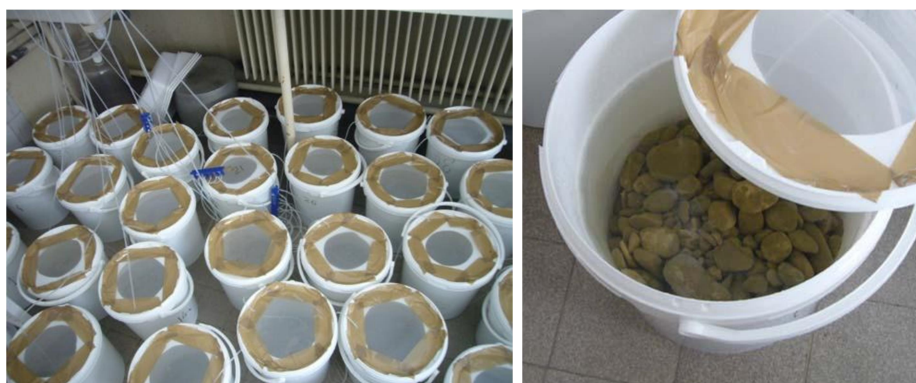
Figure 4.11 Sediment dug from dry IRES can be rehydrated with oxygenated water for 28 days to trigger the development of dormant invertebrates within the ‘seedbank’.
