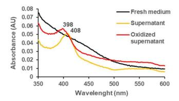
**Fig. 3** UV-visible spectrogram of *G. sulfurreducens* spent medium (0.22-μm filtered, raw or air-oxidised) after 2 days of culture compared to fresh medium
