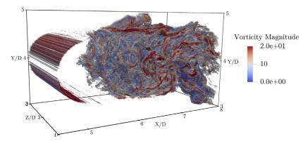
**Fig. 2.** Snapshot view of Sub-domain 2: (a), Pressure iso-surface coloured by the magnitude of pressure; (b), Lagrangian trajectories of 20,000 particles after 1000 DNS time steps coloured by the velocity magnitude; (c), Q criterion representation of the Eulerian flow structures coloured by the vorticity magnitude.
