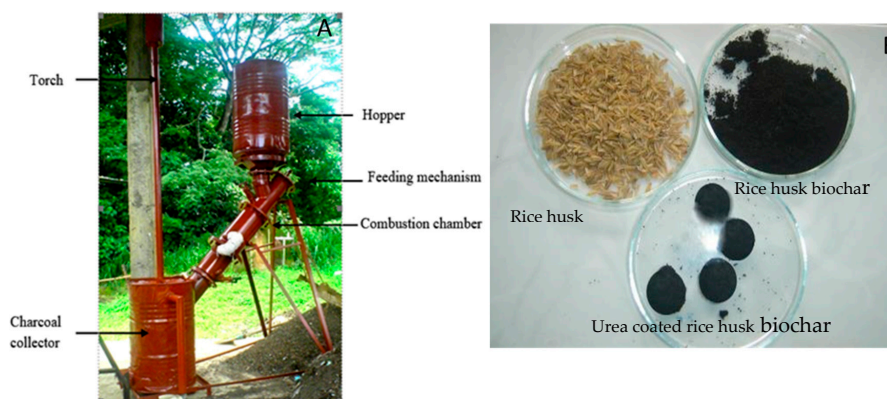
Figure 6. The material used for the biochar production and urea coated biochar generated. A. Pyrolizer; B. Slow releasing nitrogen fertilizer prepared using biochar.
