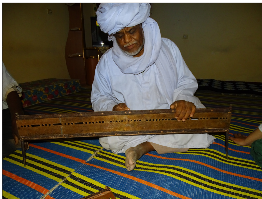
Picture 2 The flow measurement device ( louh ) is used by the water master to check the water shares of different water owners of particular foggaras (April 2017).
