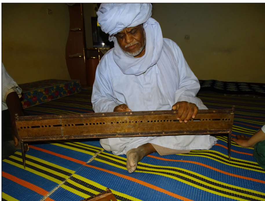
Picture 2 The flow measurement device ( louh ) is used by the water master to check the water shares of different water owners of particular foggaras (April 2017).
