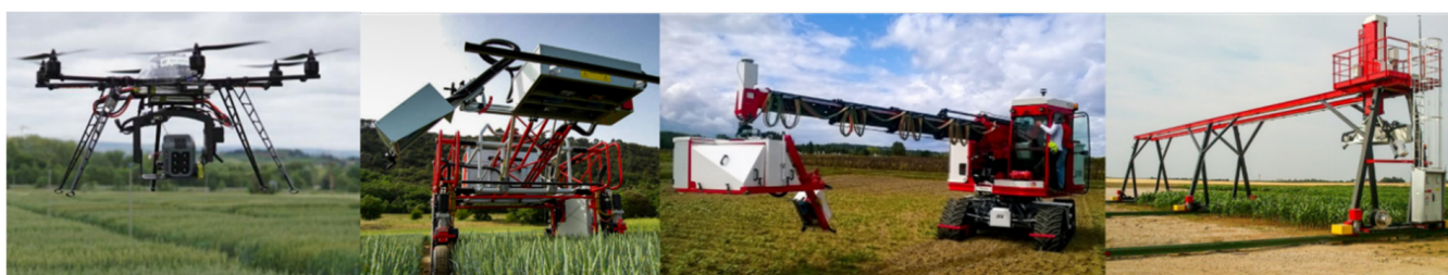
Figure 4. Different phenotyping systems used within the BREEDWHEAT project. From left to right: UAV equipped with a multispectral camera; Phenobile V1 for crops lower than 1.2 m in height; Phenobile V2 for crops up to 3 m in height; and the gantry system set up on PhenoField [95].
