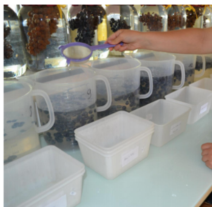
Figure 1: Picture of densimetric baths used for maturity degree sorting of grape berries.
