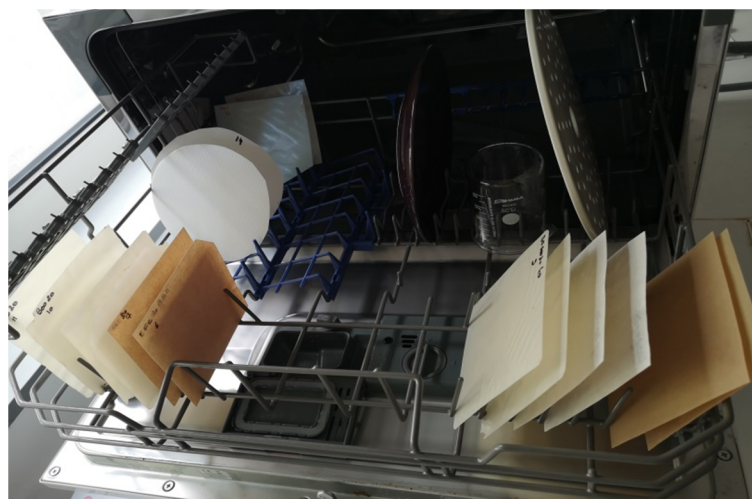
Figure 1. Dishwasher containing PHBV-based films.
