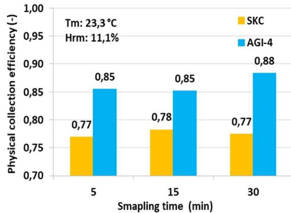
Fig. 3. Physical efficiency of impingers at different sampling times.
