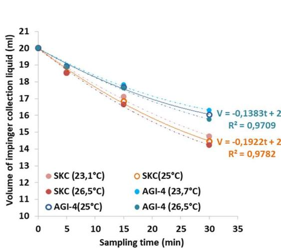
Fig. 2. Liquid evaporation/ aerosolization rate of impingers at different sampling times
