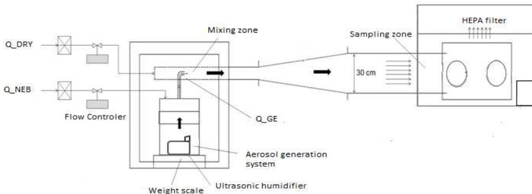
**Fig1: Schematic diagram of aerosol test system**
