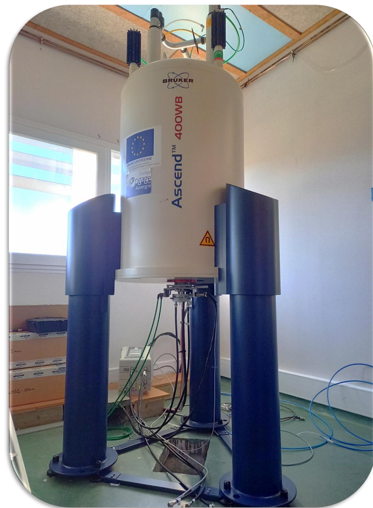
Fig 1: Picture of the equipment (Bruker Ascend 400WB with a Ø 3mm 1H/23Na volume radiofrequency antenna) and the set-up of a sample in the radiofrequency antenna.
