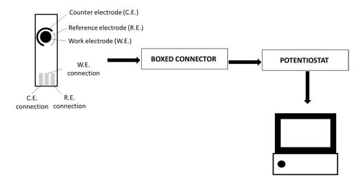
Figure 1. Cyclic voltammetry experimental set-up.
