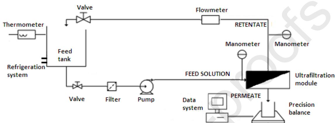
Figure 2: Schematic diagram of the ultrafiltration pilot.
