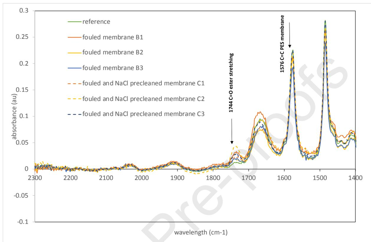
Figure 6: ATR-FTIR spectra of the clean membrane (reference), fouled membrane (B) and fouled and NaCl precleaned membrane (C).
