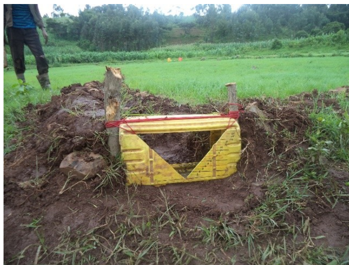
FIGURE 2 V-notch weir cut from a plastic jar allowing one to measure runoff and sediment yield in micro-catchments at low cost and low risk (at CR2).
