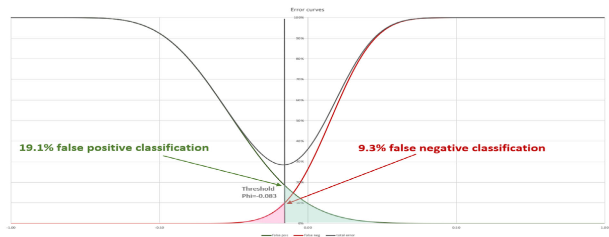
Figure 21: Distribution functions of the overall Phi-scores for negative (descending, green) and positive pest (ascending, red) estimated from the reference data set. The grey curve is the sum of both distribution functions indicating the total misclassification error. The decision rule (vertical line) minimises the total error. The crossings with the individual curves are the false-positive and false-negative classification rate
