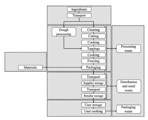
Fig. 1. Steps in pizza production considered in the LCA.
