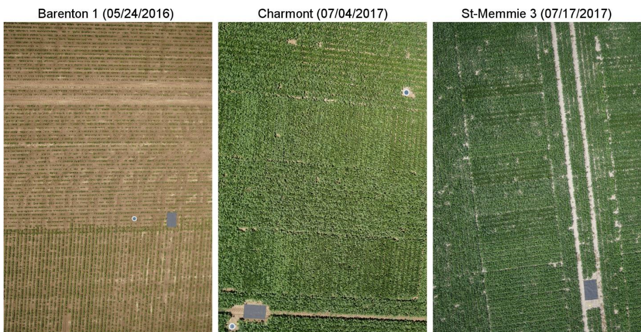
176 Fig. 1 : Examples of RGB images acquired from the UAV over three sites showing differences in growth stages, nitrogen 177 fertilizations and soil properties (Table 1). For each image, the rectangular gray panel is the reference panel used for 178 radiometric calibration, while the smaller circular panels are the GCPs used for georeferencing and orthomosaicking.
