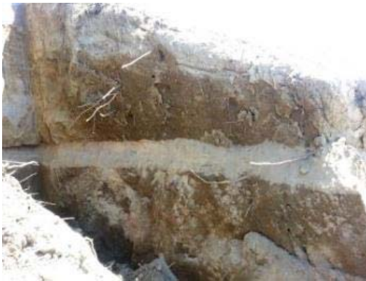
Figure 4.13 Scenario n°5: Backward erosion in a sand layer after uplift the silty blanket overlying the sandy soil strata.
