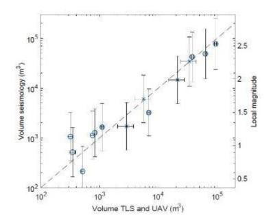
Figure 12. Volume estimated from the seismic signals and equivalent local magnitude as a function of rockfall volume estimated from TLS (circles) or UAV surveys (crosses) (summing over all events in each time interval). Error bars are 95% confidence intervals given by a linear fit of logarithms of volumes.
