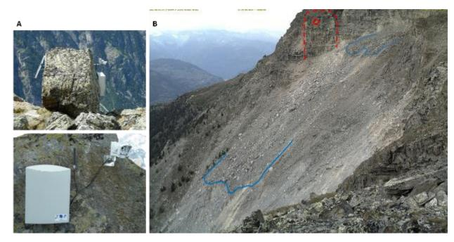
Figure 3.: Set-up of the hourly terrestrial time-lapse photography: a) the installed automatic camera on a large boulder on stable bedrock and b) example of a photograph taken by the automatic camera, displaying the situation before the summer of 2019, indicating the unstable Grosse Grabe North Pillar (striped line), the location of the small scale 2017 rockfall (red circle) and the rock glaciers (blue lines) as the initial subject of study.
