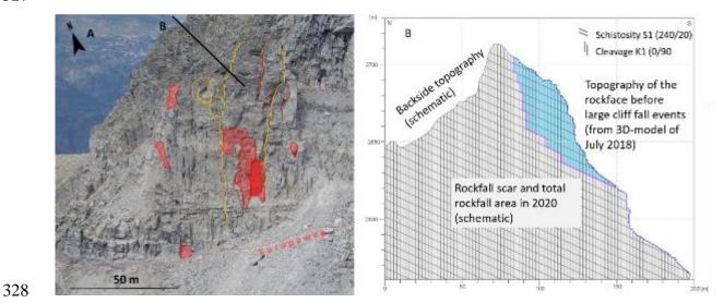
Figure 5. Close up of Grosse Grabe North Pillar: a) Before any large rockfall occurred (photograph of 06/09/2018). Precursory indicators of destabilization could already be observed by terrestrial laser scanner (red) and automatic camera (yellow) in forms of small scale rockfall (< 10<sup>3</sup> m<sup>3</sup>) and fracture opening. And b) geological cross section showing main schistosity and cleavage related to the total rockfall area and scar surface (derived from ShapeMetric3D software).
