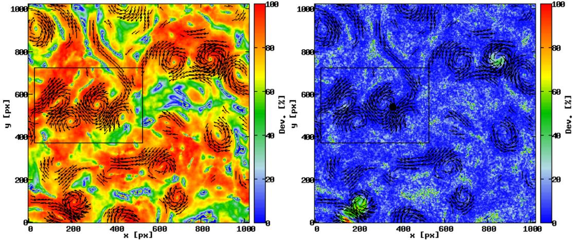
Figure 4.21: Map of color of the deviation of [Corpetti et al. \(2006\)](#) from the exact velocity modulus – Vector field of the exact solution for  $\|\mathbf{u}\|/\|\mathbf{u}\|_{\max} > 30\%$ . Top: PSNR = 12 dB; Bottom, PSNR = 24 dB.
