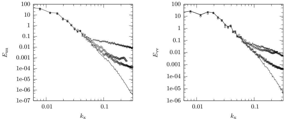
Figure 4.13: Spectra of the velocity extracted from images of particles (case C1a FLUID project database) with: (-), DNS; (+), **OF1** approach; ( $\square$ ), **OF2** approach; ( $\circ$ ) correlation technique.
