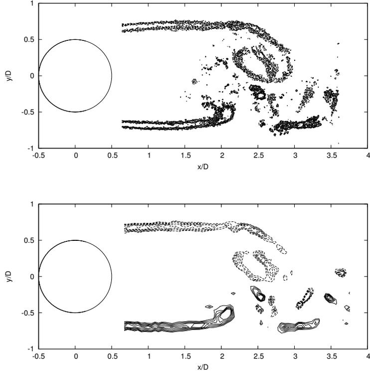
Figure 4.6: View of instantaneous near wake iso-contour of vorticity at  $Re=3000 - \omega_z^* = (\omega_z U)/D$  ( $|\omega_{z_{\min}}^*| = 0.5$ ,  $|\omega_{z_{\max}}^*| = 10$ ,  $\Delta\omega_z^* = 1$ ): Top, Optical-flow treatment; Bottom, PIV treatment.
