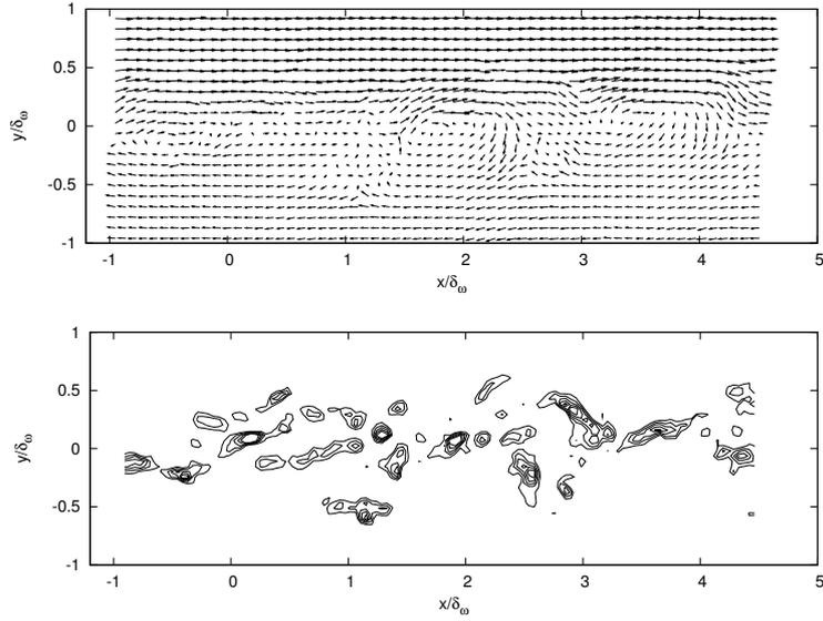
Figure 4.3: Views of instantaneous turbulent plane mixing layer structure at  $Re_{\delta_\omega} = 7000$ . PIV - multipass 32-16 treatment: Top, Instantaneous vector field (one vector out of nine); Bottom, Instantaneous spanwise isocontour of vorticity  $\omega_z^* = (\omega_z \Delta U) / \delta_\omega$  ( $\omega_{z_{\min}}^* = -9$ ,  $\omega_{z_{\max}}^* = -2$ ,  $\Delta\omega_z^* = 1$ ).
