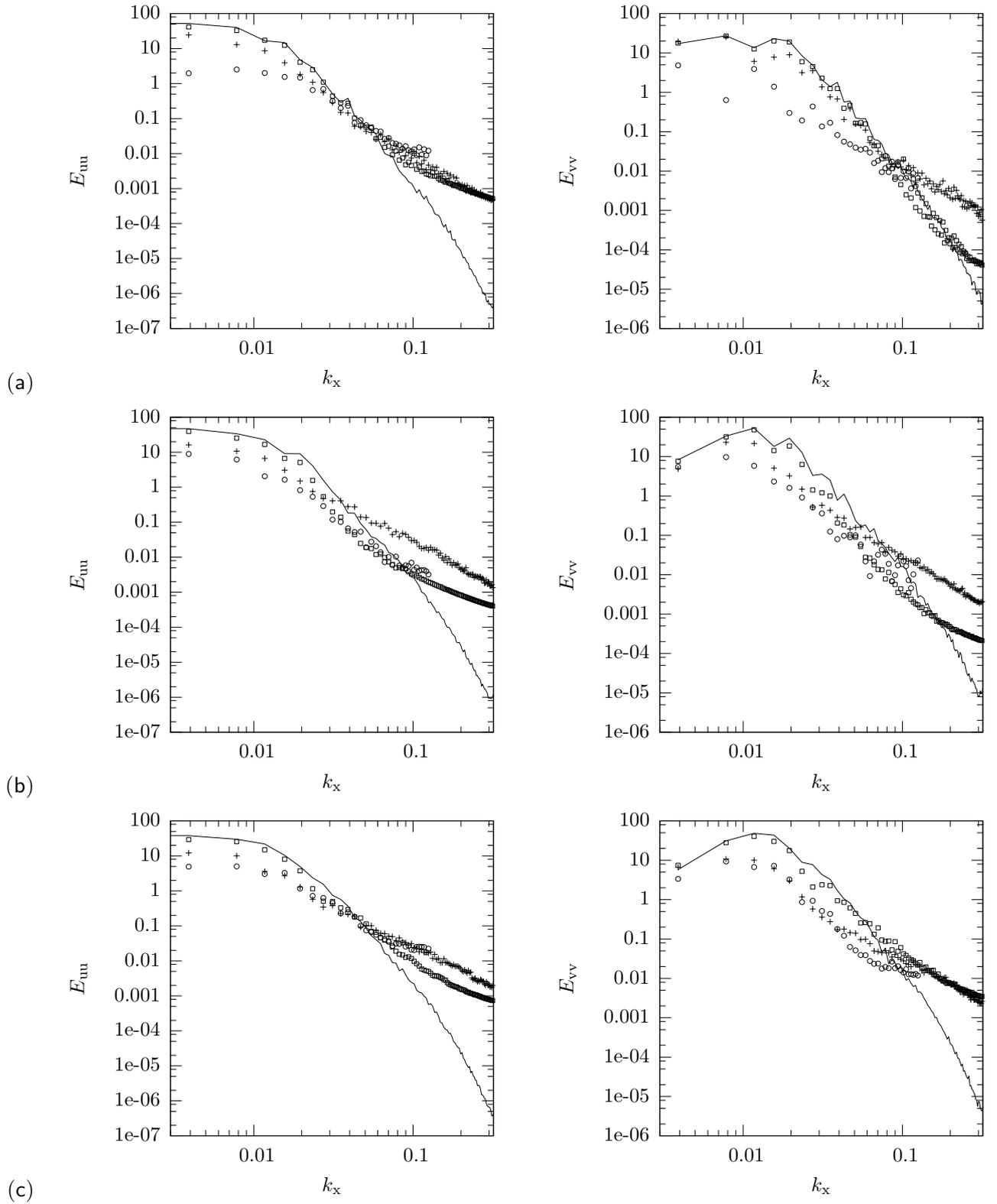
Figure 4.17: Spectra of the velocity extracted from images of scalar (case C1b FLUID project database) with: (-), DNS; (+), OF1 approach; ( $\square$ ), OF2 approach; ( $\diamond$ ), correlation technique; at three time steps: (a),  $t = 0\Delta t$ ; (b),  $t = 640\Delta t$ ; (c),  $t = 1000\Delta t$ .
