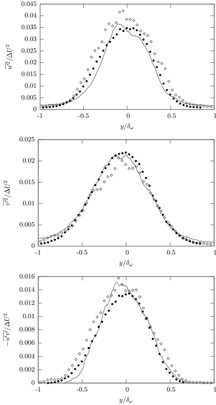
Figure 4.4: Reynolds stress distributions of the mixing layer at  $x/\delta_\omega = 4$ . Each symbol representing a velocity measurement technique: —, Optical-flow;  $\diamond$ , PIV;  $\bullet$ , Hot-wire (Heitz, 1999).
