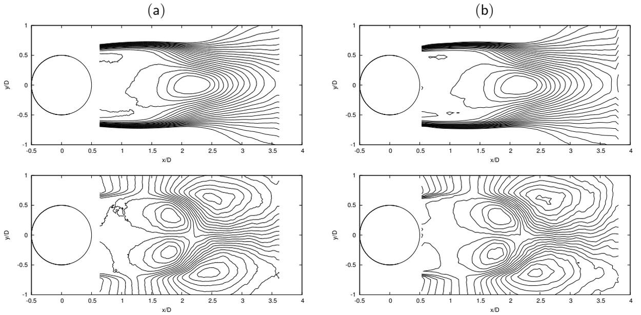
Figure 4.7: From top to bottom, 21 iso-contours of mean streamwise velocity  $U/U_\infty = -0.2, \dots, 1$  and of mean transverse velocity  $V/U_\infty = -0.25, \dots, 0.25$ : (a), Optical-Flow measurements; (b), PIV measurements.
