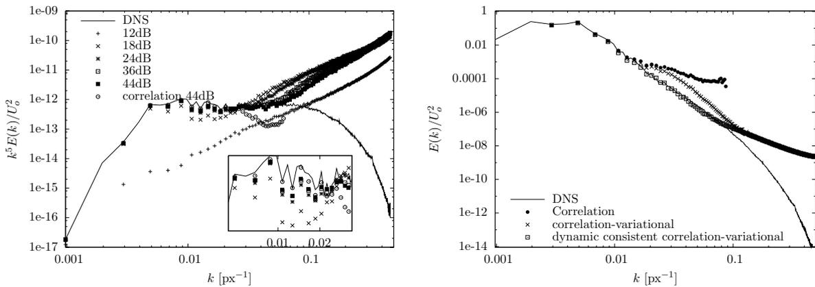
Figure 4.22: Compensated energy spectra: Left, multiresolution approach of [Corpetti et al. \(2006\)](#) for different levels of noise in the images; Right, Comparisons between different approaches for PSNR=12dB.
