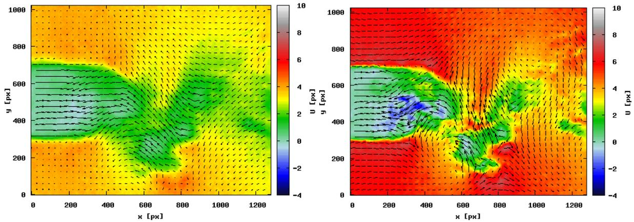
Figure 4.24: Instantaneous vector field with horizontal velocity color map, in near the wake of a circular cylinder at  $Re = 3900$ . Left, optical-flow approach (Corpetti *et al.*, 2006); Right, COROF1 collaborative approach.
