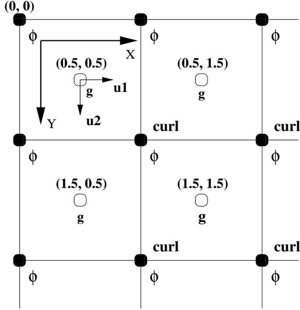
Figure 3.1: Definition of finite-dimensional spaces of scalar fields and vector fields on a square grid. Filled circles depict *nodes* or *vertices*, the other circles indicate *cells*. The positions of diamonds are referred to as *sides*.
