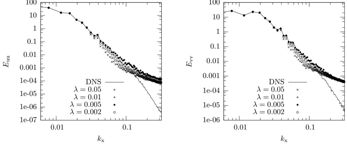
Figure 4.18: Influence of the regularization parameter  $\lambda$  on the spectrum of the vertical velocity component estimated with **OF2** method – 2D turbulent flow (case C1a).
