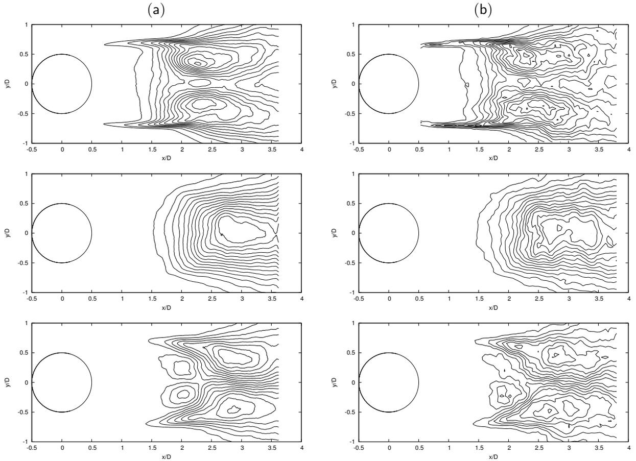
Figure 4.8: From top to bottom, 15 iso-contours of  $\overline{u'^2}/U_\infty^2 = 0, \dots, 0.05$ ,  $\overline{v'^2}/U_\infty^2 = 0, \dots, 0.1$  and  $\overline{u'v'}/U_\infty^2 = -0.025, \dots, 0.025$ : (a), Optical-Flow measurements; (b), PIV measurements.
