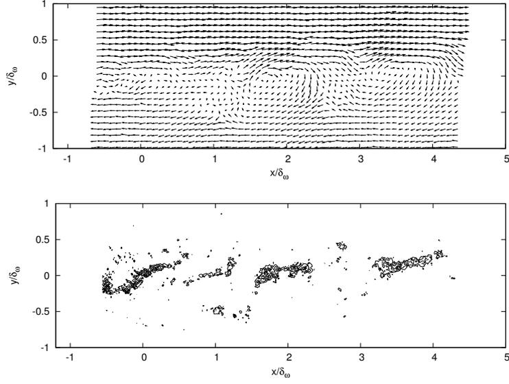
Figure 4.2: Views of instantaneous turbulent plane mixing layer structure at  $Re_{\delta_\omega} = 7000$ . Optical-flow: Top, Instantaneous vector field (one vector out of 225); Bottom, Instantaneous spanwise isocontour of vorticity  $\omega_z^* = (\omega_z \Delta U) / \delta_\omega$  ( $\omega_{z_{\min}}^* = -9$ ,  $\omega_{z_{\max}}^* = -2$ ,  $\Delta\omega_z^* = 1$ ).
