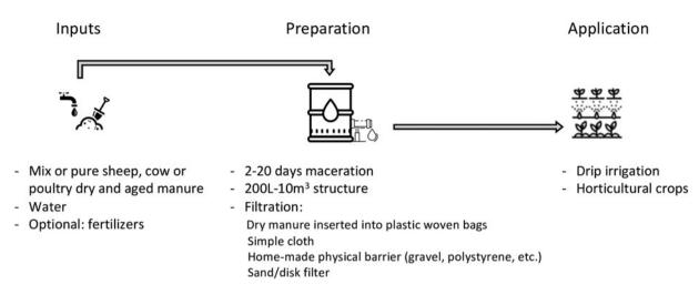
Fig. 2. Homemade dry manure-based tea production protocol.
