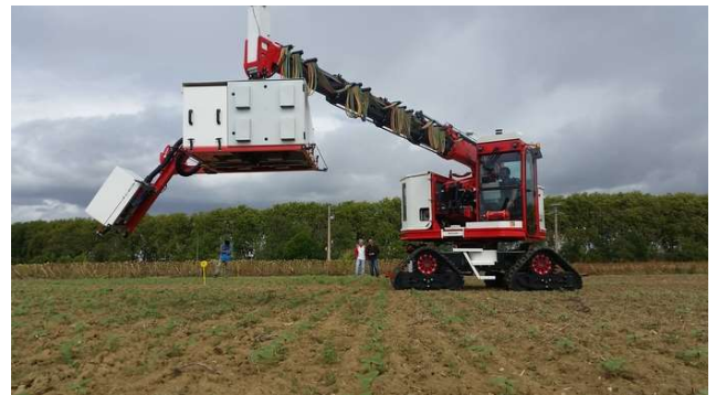
Figure 1. The phenomobile with caterpillars showing the 12m long boom supporting the measurement head.
