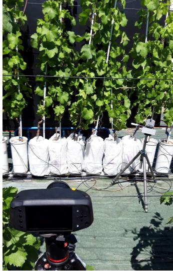
Figure 3: Typical scene where hyperspectral images were acquired. One image corresponded to one of the modalities of the experimental design with 6 pots of vines. The reference is placed in the scene.
