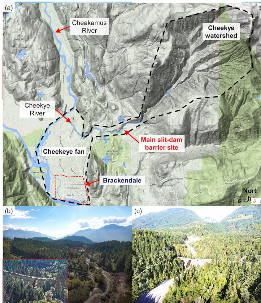
**Figure 7.** The proposed Cheekye slit-dam. (a) Map of the surrounding region; (b) rear view; (c) front view. Note that the dam has been digitally added to (b) and (c).
