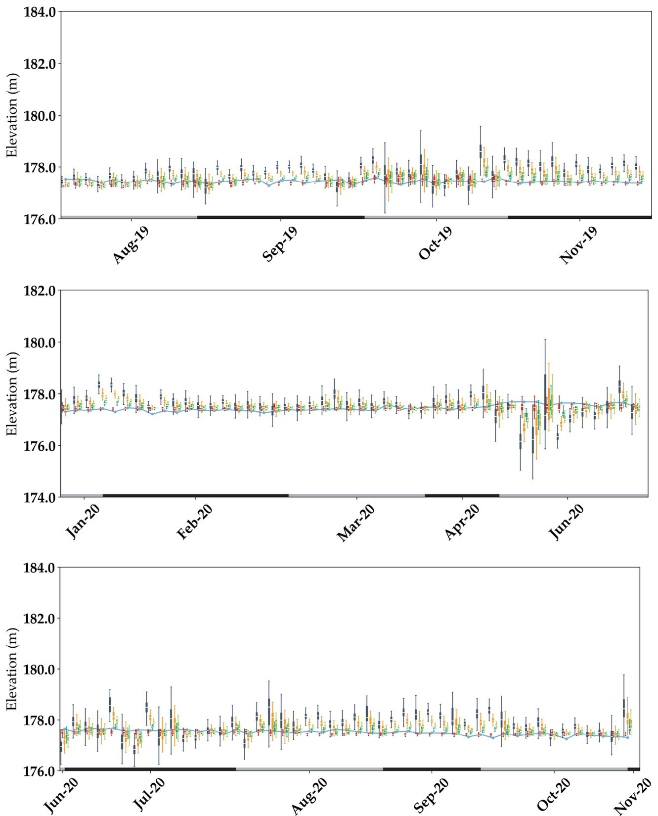
**Figure A4.** Boxplot by track of the original estimated elevations by GEDI over Lake Michigan and the four tested models presented in Sections 3.1.1 and 3.1.2. The blue line represents in situ elevations.
