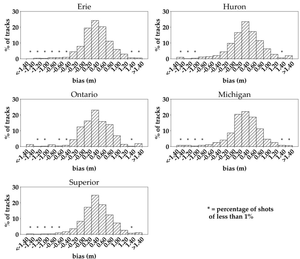
**Figure 4.** Distribution of the mean difference (bias) between GEDI shots and in situ elevations across the five studied lakes. Biases correspond to the mean difference calculated for a given track (GEDI shots acquired on a given date with a given beam).
