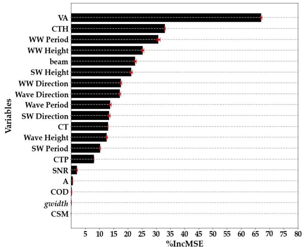
**Figure A11.** Variables' order of importance in the error estimation random forest regression model with the percentage mean increase in MSE (%IncMSE) (higher values mean higher importance). WW represents wind generated waves variables. SW represents swell waves variables.
