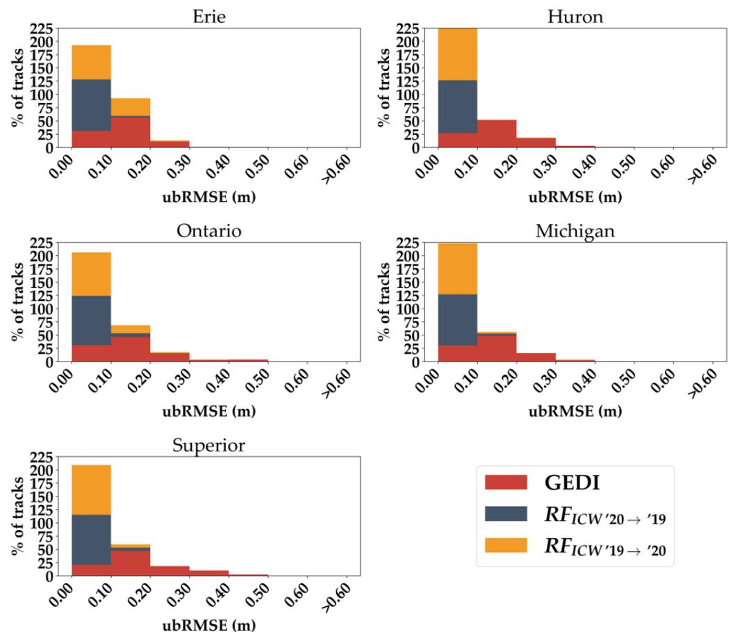
**Figure 9.** Stacked histograms of the distribution of the unbiased root mean squared error (ubRMSE) between GEDI (resp.  $RF_{ICW}$  '19→'20 and  $RF_{ICW}$  '20→'19) and in situ elevations across the five studied lakes. The distribution corresponds to the ubRMSE of GEDI shots grouped by acquisition date and the acquiring beam.  $RF_{ICW}$  '19→'20 (resp.  $RF_{ICW}$  '20→'19) corresponds to the  $RF_{ICW}$  model, trained over 2019 (resp. 2020) data and validated on 2020 data (resp. 2019).
