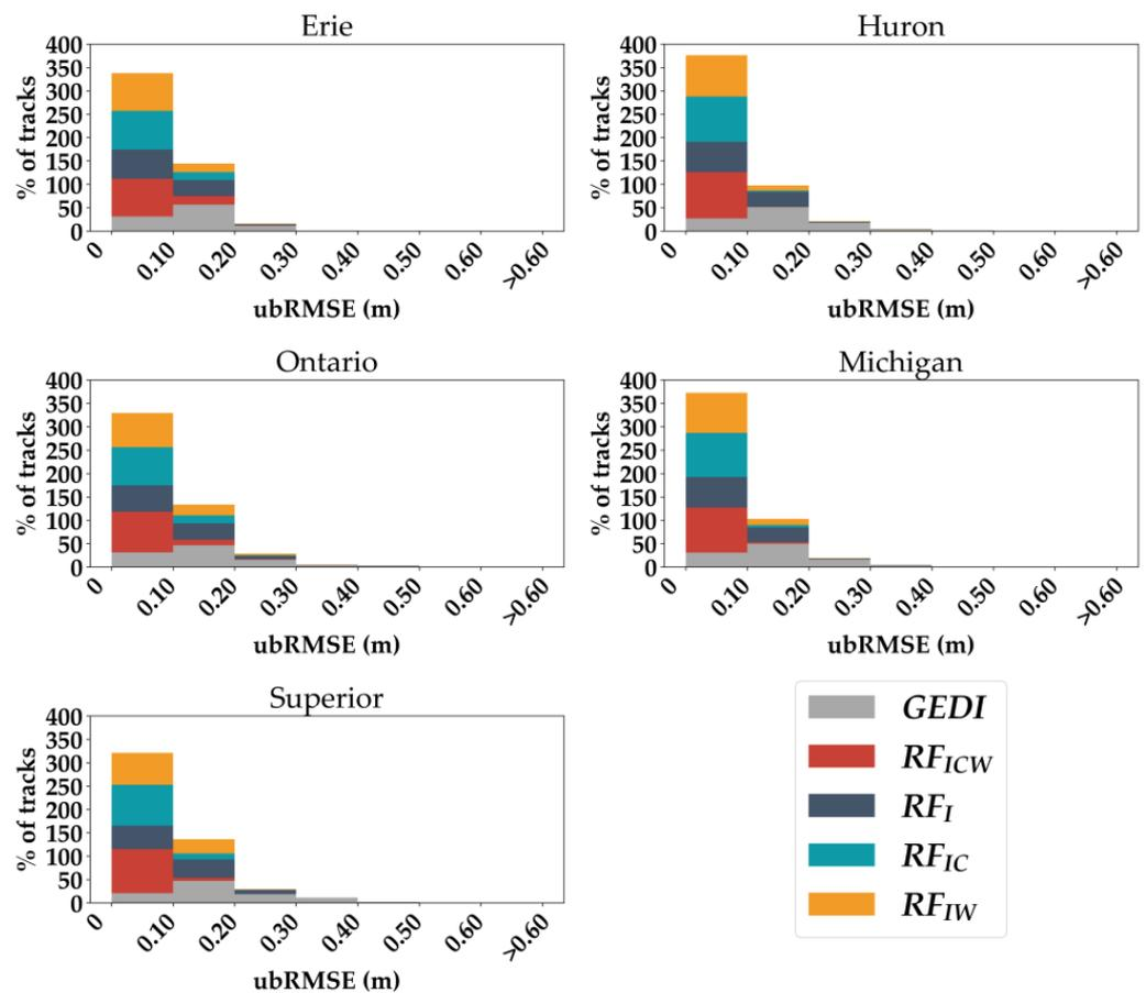
**Figure 12.** Stacked histograms of the distribution of the unbiased root mean squared error (ubRMSE) between GEDI (resp.  $RF_{ICW}$ ,  $RF_I$ ,  $RF_{IC}$ , and  $RF_{IW}$ ) and in situ elevations across the five studied lakes. The distribution corresponds to the ubRMSE of GEDI shots grouped by acquisition date and the acquiring beam.
