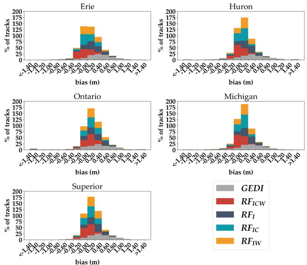
**Figure 11.** Stacked histograms of the distribution of the mean difference (bias) between GEDI (resp.  $RF_{ICW}$ ,  $RF_I$ ,  $RF_{IC}$ , and  $RF_{IW}$ ) and in situ elevations across the five studied lakes. Biases correspond to the mean difference calculated for GEDI shots grouped by acquisition date and the acquiring beam.
