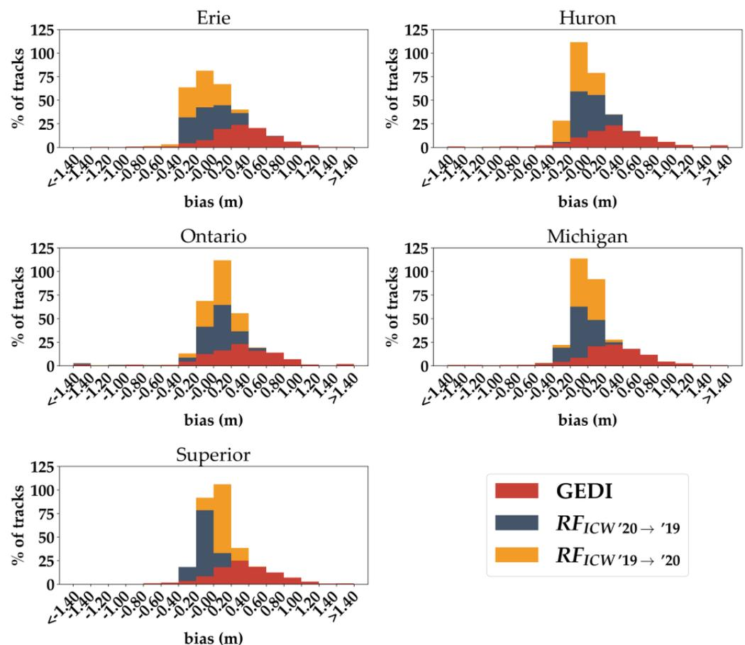
**Figure 8.** Stacked histograms of the distribution of the mean difference (bias) between GEDI (resp.  $RF_{ICW}$  '19→'20 and  $RF_{ICW}$  '20→'19) and in situ elevations across the five studied lakes. Biases correspond to the mean difference calculated for GEDI shots grouped by acquisition date and the acquiring beam.  $RF_{ICW}$  '19→'20 (resp.  $RF_{ICW}$  '20→'19) corresponds to the  $RF_{ICW}$  model, trained over 2019 (resp. 2020) data and validated on 2020 data (resp. 2019).
