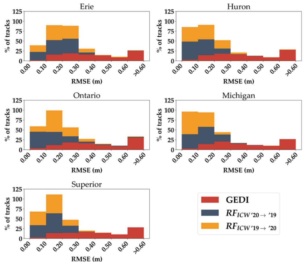
**Figure 10.** Stacked histograms of the distribution of the root mean squared error (RMSE) between GEDI (resp.  $RF_{ICW}$  '19→'20 and  $RF_{ICW}$  '20→'19) and in situ elevations across the five studied lakes. The distribution corresponds to the RMSE of GEDI shots grouped by acquisition date and the acquiring beam.  $RF_{ICW}$  '19→'20 (resp.  $RF_{ICW}$  '20→'19) corresponds to the  $RF_{ICW}$  model, trained over 2019 (resp. 2020) data and validated on 2020 data (resp. 2019).
