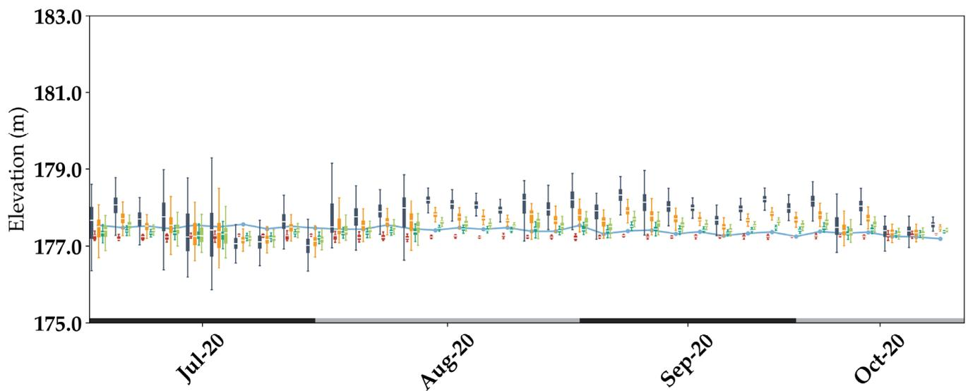
**Figure 7.** Boxplot by track of the original estimated elevations by GEDI over Lake Huron and the four tested models presented in Sections 3.1.1 and 3.1.2. The blue line represents in situ elevations.
