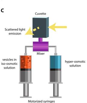
Fig. 2 Illustrations of measurements of hydraulic properties at the cell level. A: drawing of a cell pressure probe, B: example pictures of protoplast before (left pictures) and after a hypo-osmotic shock (pipette diameter  $\sim\!10~\mu\text{m}$ ), C: drawing of a stopped-flow spectrophotometer
