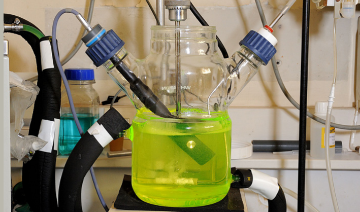
Dircom Cnam ©Sandrine Villain - Determination of the oxygen transfer coefficient in a bioreactor
