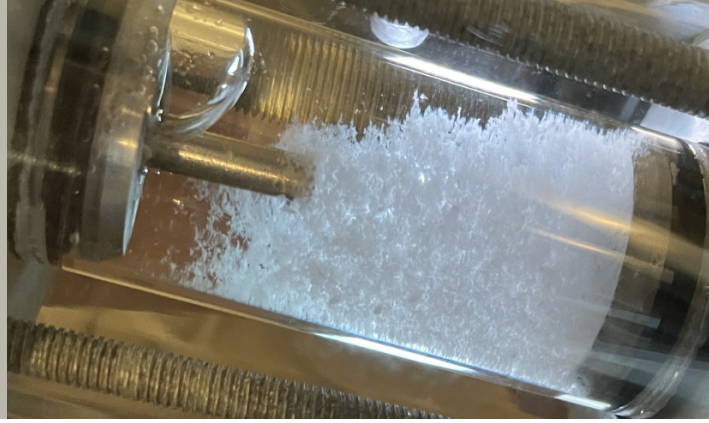
©Nada Chami - Appearance of a mixed CP/CO 2 hydrate slurry
