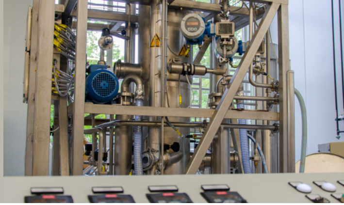
©Éric beaumont, INRAE - Pilot evaporator of the dairy platform at the Joint Research Centre for Science and Technology of Milk and Eggs (UMR STLO) in Rennes .
