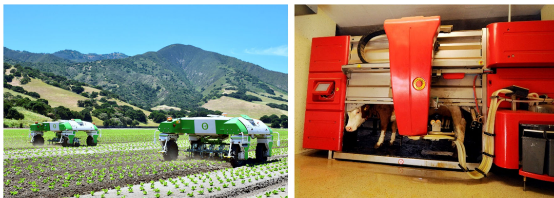
Fig. 1 Left: weeding robot for vegetable production, photo by Naïo Technologie; right: automated milking system, iStock photo by Elmar Gubisch
