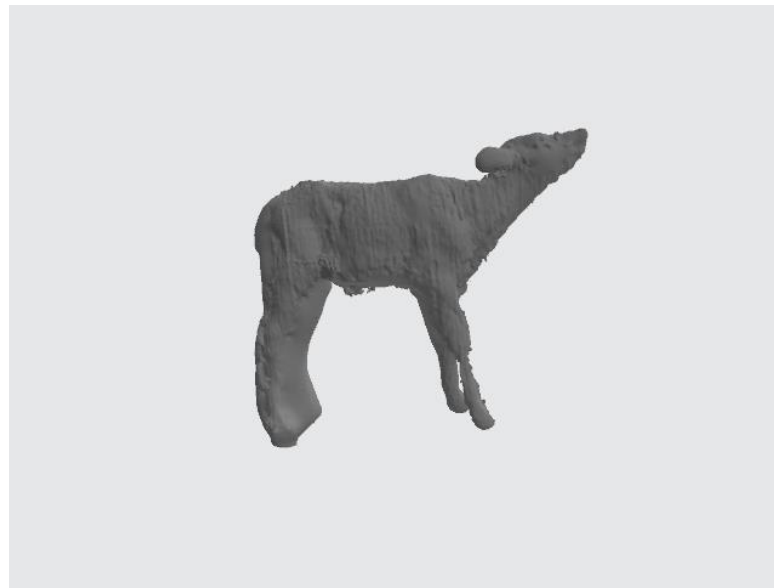
Figure 1. Abnormal image representing the presence of a “skirt” on the legs. When the number of points is insufficient, the software fills in the volume between the points located on different legs (which is not the case when there are enough points).
