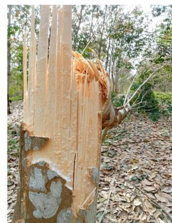
Figure 2: Trunk breakage of a 6-year-old rubber tree after bending test.
