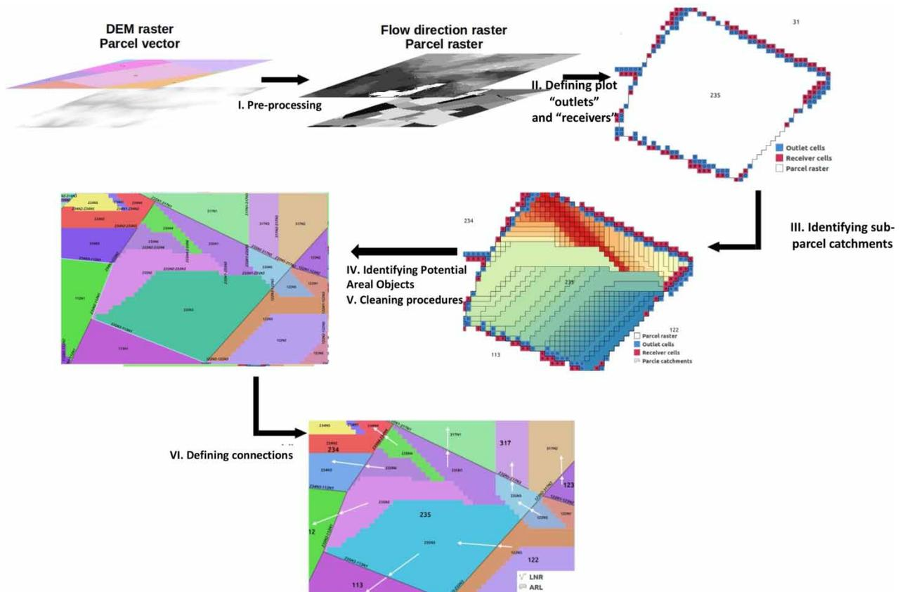
**Figure 1** | Steps for building an oriented tree of areal and linear features.
