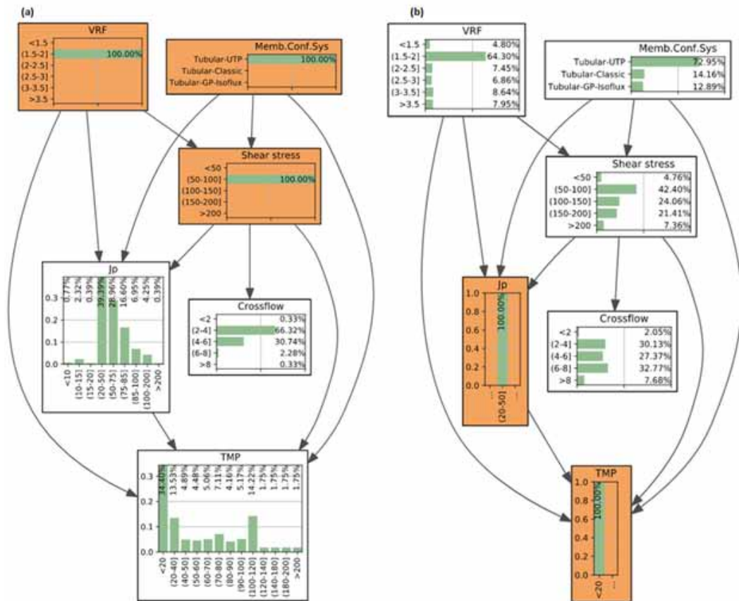
Figure 6. (a) Estimated probability distributions of the transmembrane pressure (TMP) and permeation flux (Jp) (green bars in white boxes) given the evidence (green bars in orange boxes). (b) Estimated probability distributions of the shear stress and volume reduction factor (VRF) constraints (white boxes) given the Jp and TMP (orange boxes).
