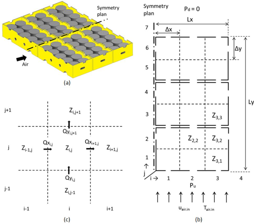
Figure 2: Pallet layer:(a) 3D view of the layer; (b) 2D zonal model; (c) zoom of zone  $Z_{i,j}$
