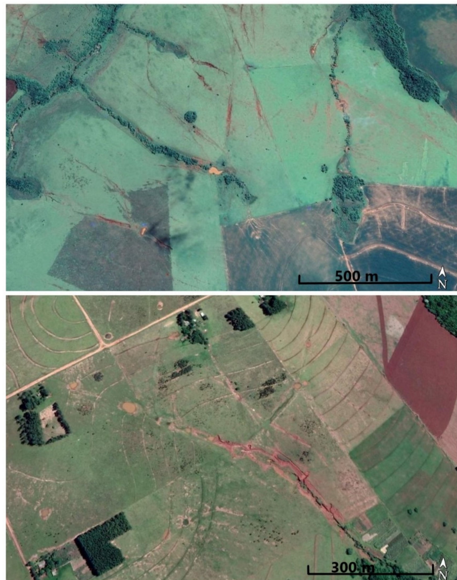
Figure 12. Examples of gullies originating near artificial reservoirs.
