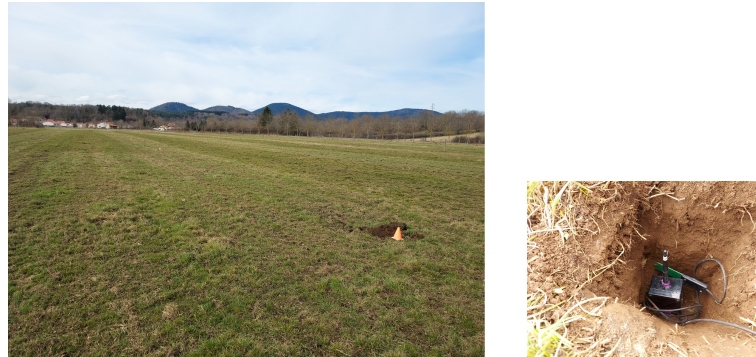
Figure 13. Experimental field (45°42'25.99" N, 3°00'40.54" E, 433 m) and a sensor node buried at 15 cm deep. Once the sensor node is installed, some soil is added and compacted by foot.
