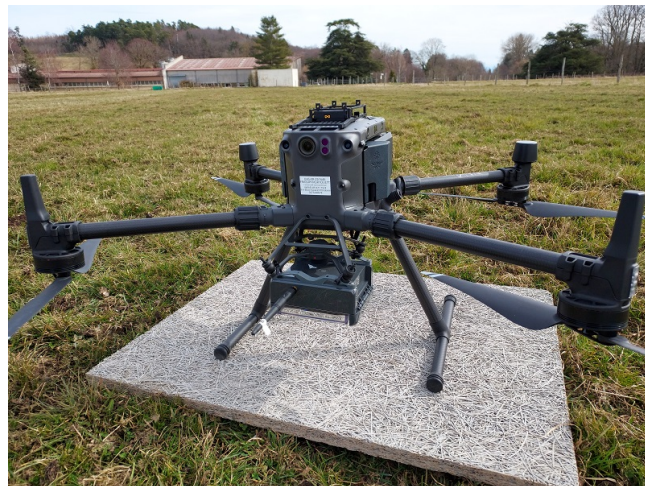
Figure 8. The UAV used for the experimentations (Matrice 300 RTK—DJI) with the collector node attached on the underside.
