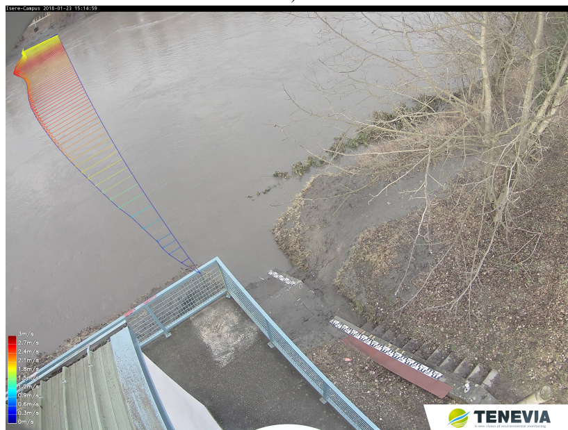
Figure 3: Surface fluid velocities extracted from surface video images on the 23/01/2018 for a stage of H = 4.03 m. a): raw PTV surface velocity vectors; b): estimated streamwise velocity profile. Color-bars are on the left of the images. River flowing from right to left and camera on the left bank.
