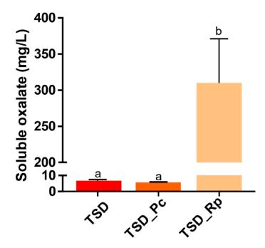
**Figure 3.** Soluble oxalate quantification in the liquid phase of the microcosm after 10-day culture of *P. chrysosporium* and *R. placenta* with TSD (TSD\_Pc/TSD\_Rp). TSD represents the control without fungus (mean  $\pm$  s.e., n = 3, one-way ANOVA and Tukey's post hoc test (*p*-value  $\leq 0.05$ ), different letters to show statistically significant differences).
