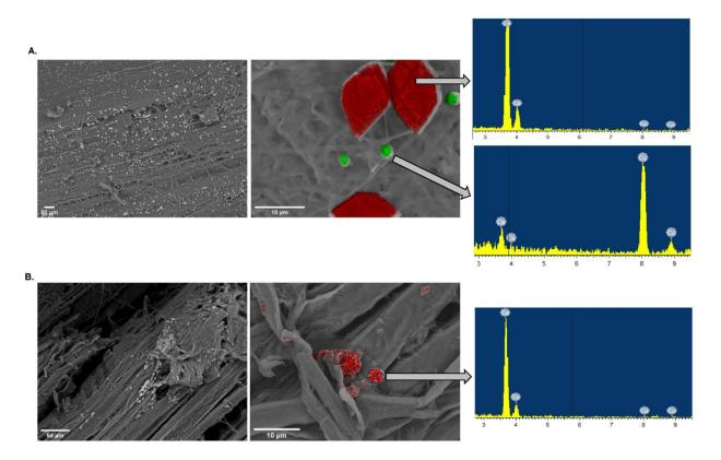
**Figure 5.** SEM images of oxalate crystals after 10-day culture of *P. chrysosporium* and *R. placenta* with TSD. (**A**) Oxalate crystals produced by *R. placenta*. Red crystals (diamond shape) and green crystals (ball shape) represent calcium and copper oxalate crystals, respectively. (**B**) Oxalate crystals produced by *P. chrysosporium*. Only calcium oxalate crystals were detected.
