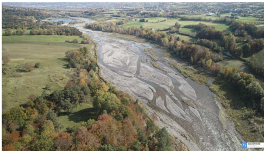
Fig. 14. Drone view of the restored reach of the Upper Drac in 2018, showing the spontaneous recovery of the braided channel morphology (@SIGosphere)
